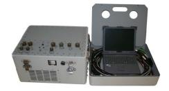
**Support Equipment** for the Terma pylon versions, Pylon EW tester (PEWT).
