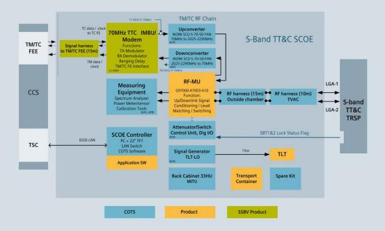
Terma's TT&C SCOE (Telemetry, Tracking & Control-Specific Check-Out Equipment) for testing the satellite platform TT&C subsystem or, at unit level, the transponder (comprising a Telecommand Receiver and Telemetry Transmitter), is based on commercial off-the-shelf (COTS) instruments and a 70 MHz IF TTC modem (IMBU: IF Modem and Baseband Unit), and has been designed for highly- accurate automated measurements.
